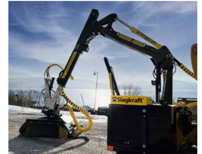
SC7 • A modern crane with a high crane pillar, short main boom and protected hoses. For clearing minor roads.
