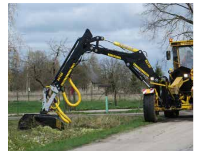
SC160 • A robust crane with a long reach of up to 11 metres with double-telescope technology. For clearing major road networks.
